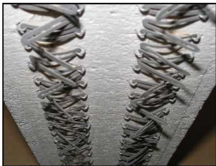
Pinned elements after high temperature cycling
