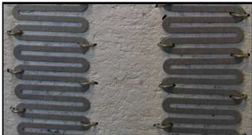
Pinned elements before high temperature cycling
