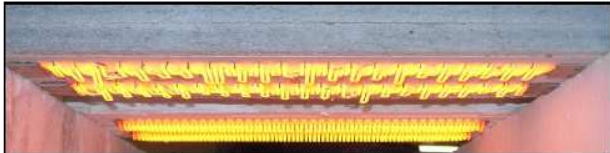
Pinned element beginning to distort
