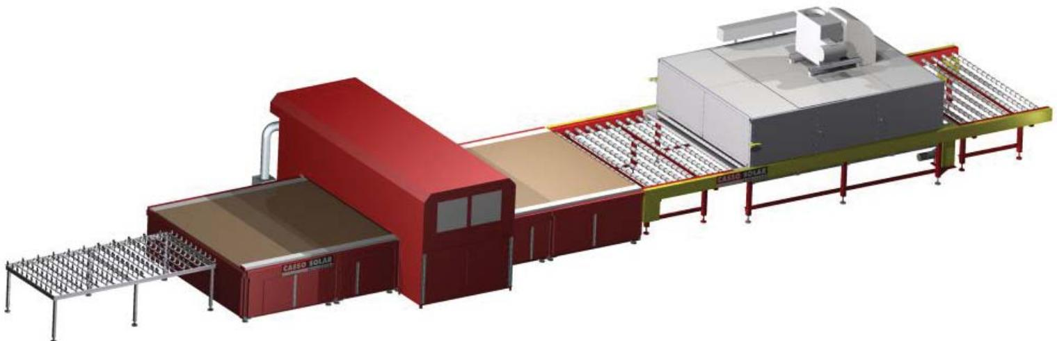
Casso-Solar Technologies Fully Automatic Spray Coating System for Glass At 6 FPM
